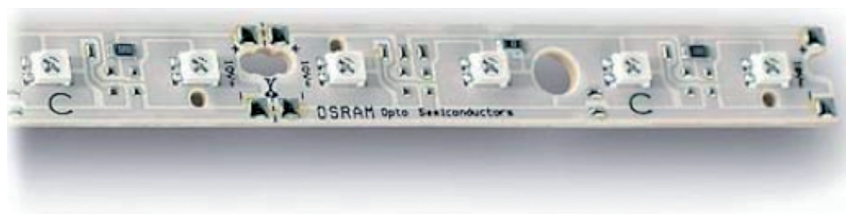
Part of an OSRAM LINEARlight Colormix module. The discrete surface mount LEDs are the white rectangular components.
